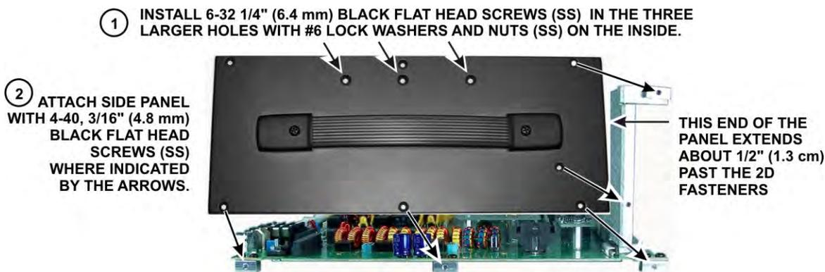
Figure 16. Mounting Left Side Panel.
