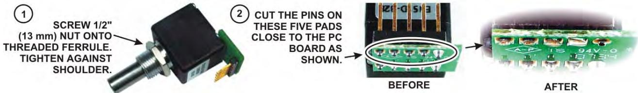
Figure 43. VFO B Encoder Assembly Preparation for Installation.
