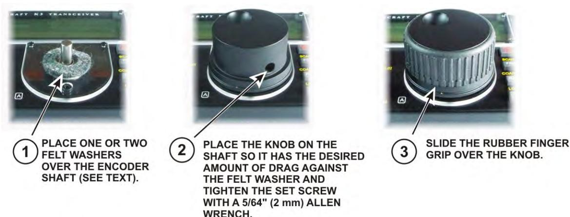
Figure 49. Mounting the VFO A Tuning Knob.
