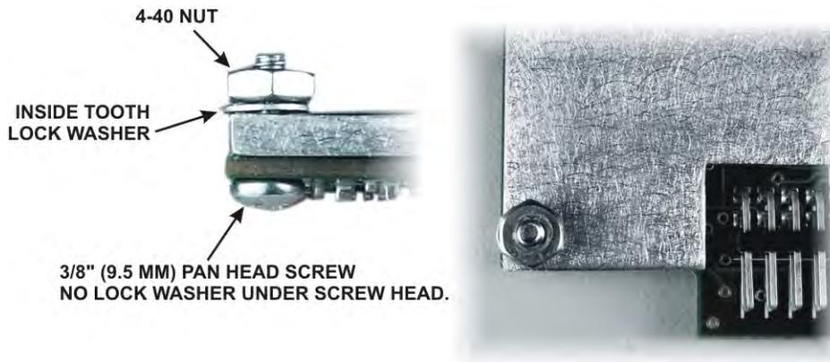
Figure 71 Stiffener Fastener on KSYN3 Board.
