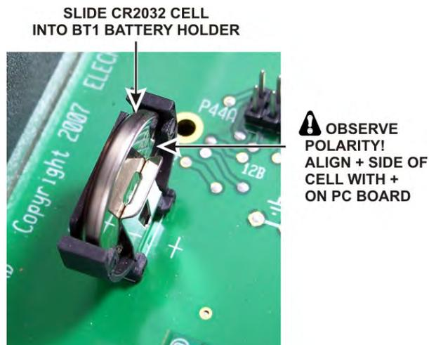
Figure 87. Installing BT1.
