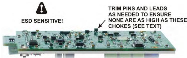
Figure 72. Checking Lead Lengths on KSYN3 Board.
