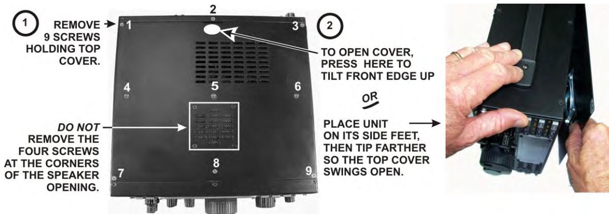
Figure 94. How to Remove the Top Cover.
