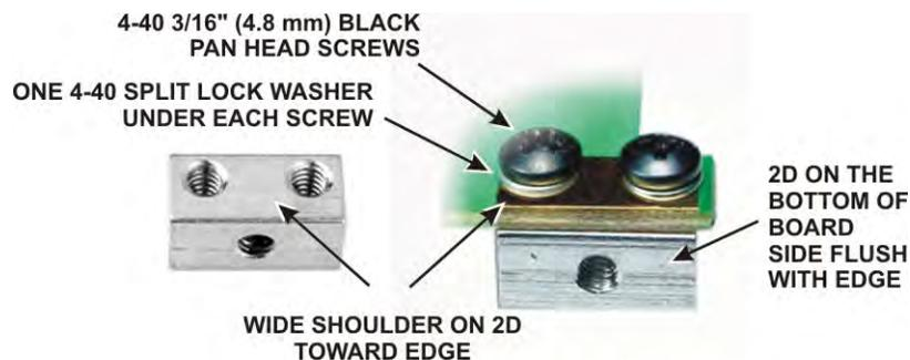
Figure 6. Installing 2D Fasteners on RF Board.
