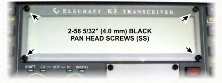
Figure 46. Installing LCD Cover.
