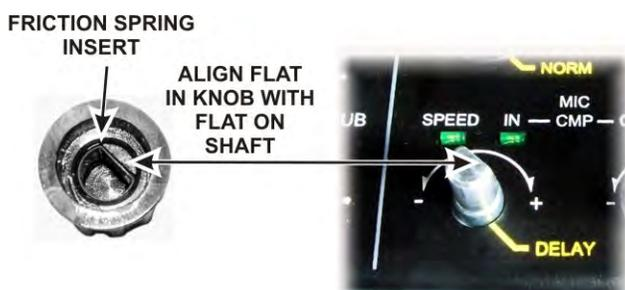
Figure 48. Mounting Friction Knobs.
