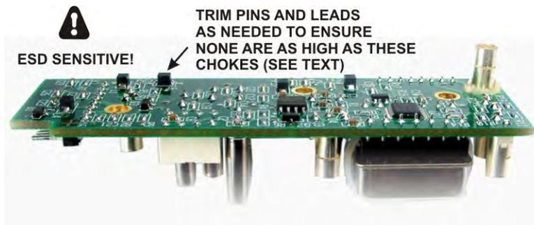
Figure 69. Checking Lead Lengths on KREF3 Board.
