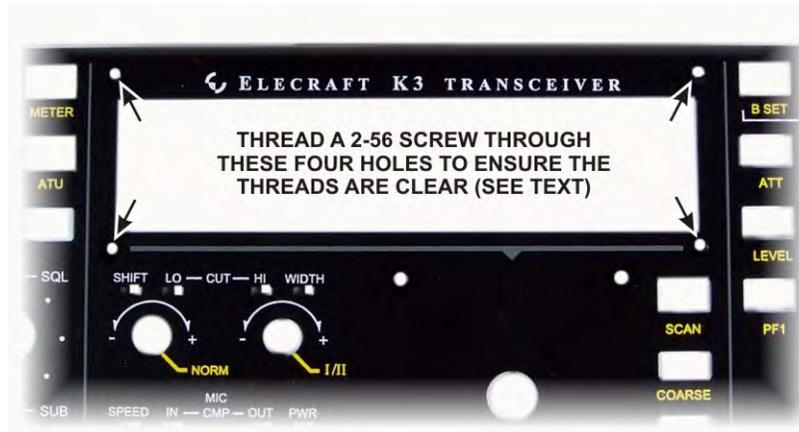
Figure 39. Checking 2-56 Threaded Screw Holes.
