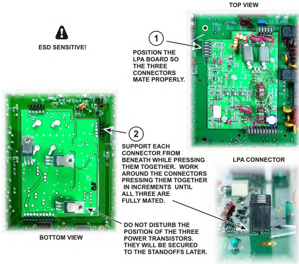
Figure 12. Installing the Low Power Amplifier (LPA).
