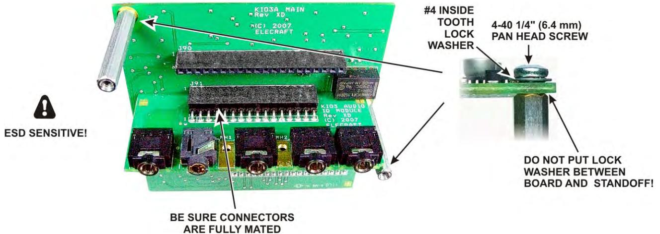
Figure 32. Preparing the KIO3 Board for Installation.
