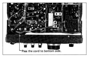
3. Turn the set upside down. Then insert the 8-P connector into J10 of the LOGIC unit.
