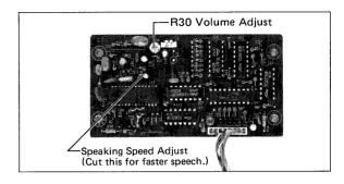
When finished with the adjustment, replace the top and bottom covers of the set.
