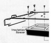
3 Pass the DC power cable atta AC power socket plate as sh the bushing into the hole. Attach the AC power socke attached the PLATE (A) bef ①, so that the AC power sock
