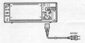
3. By turning the transceiver power switch ON, this unit will be turned ON and supply a DC 13.8V to the transceiver.
