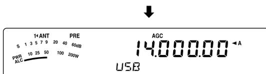
❸ Confirm that VFO A has been selected for communications; "◀A" should be visible on the display. If it has not, press [A/B / M/V] to select VFO A.
