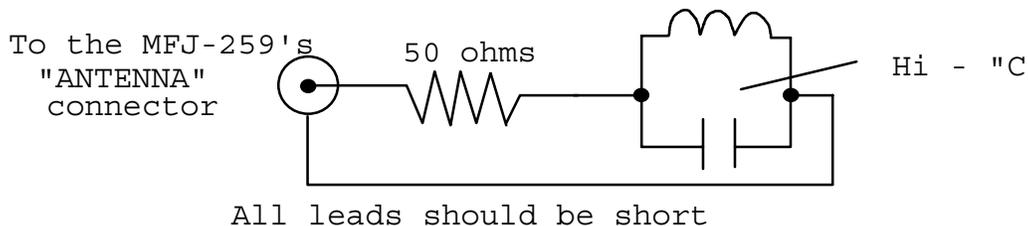
For high inductance values a series LC circuit should be used to measure resonant frequency. The inductor and capacitor should be connected in series through a 50Ω low inductance carbon resistor across the "ANTENNA" connector on the MFJ-259.
