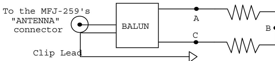
A properly designed current balun, the type that is the most effective and usually handles the most power, should show a low SWR over the entire operating range of the balun with the clip lead in any of the three positions.
