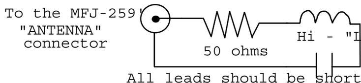
Tune the MFJ-259's frequency until the "SWR" meter reaches the lowest SWR. This is the resonant frequency of the load.
