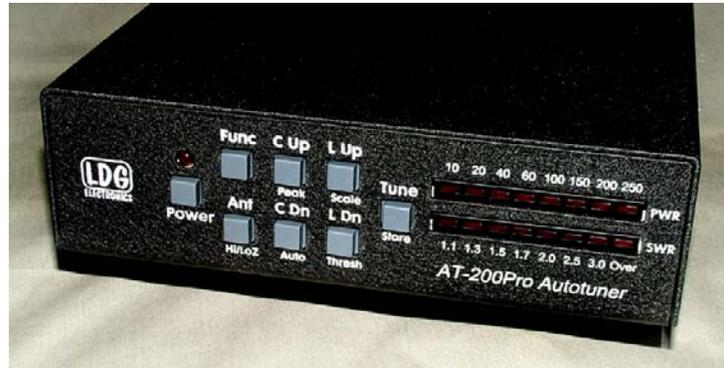
The front panel presents seven pushbutton controls, and two LED meters:
