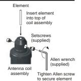
Note: Installation of the ATAS-120 on a hatchback or trunk lid may not permit a low SWR to be obtained. A solid bond to the car body is important so as to establish a counterpoise for the vertical radiating element.
