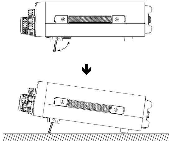
**Note:** Do not use the wire stand as a carrying handle, as it could slip out of its mount, causing the transceiver to be dropped! Use the carrying handle on the side of the FT-847 for transport purposes.
