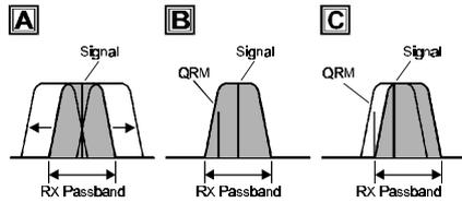
This feature is operational in all modes except FM, although the effect in the AM mode may not be dramatic due to the wider bandwidth used during AM operation. The **SHIFT** control's function is dedicated to the receive mode, and does not affect your transmitted signal characteristics; such adjustment of the transmitted signal is, however, provided via Menu items #92 and 93, as described on page 90.
