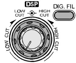
To activate the DSP passband filter, press the [**DIG. FIL**] switch; the "DIG. FIL" icon will appear on the display when the DSP is on. Now rotate the **HIGH CUT** and **LOW CUT** controls to roll off interference and/or noise, as needed, or to enhance the audio response. Press the [**DIG. FIL**] switch again to turn the DSP passband filter off.
