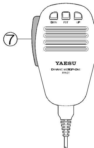
**Note:** In step ⑦ above, pressing the **PTT** switch does *not* activate the transmitter. It simply sends a signal to the microprocessor that an independent *Transmit* frequency is being stored on the same channel as a previously-stored *Receive* frequency.
