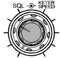
When a signal is received which exceeds the threshold set by the **SQL** control, the muting function will be disabled and normal receiver audio will flow. When the signal disappears, the receiver will again be muted.
