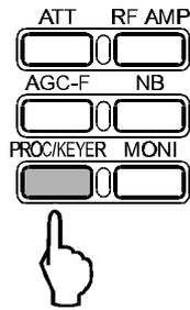
**Note:** The RF SPEECH PROCESSOR is disabled during *Satellite* operation.
