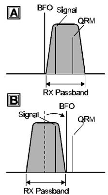
**Note:** When sidebands are switched, all aspects of CW operation are switched at once, including the transmitted CW carrier and the displayed frequency. This avoids the necessity of making multiple adjustments so as to align the receiver and transmitter sections for proper operation.
