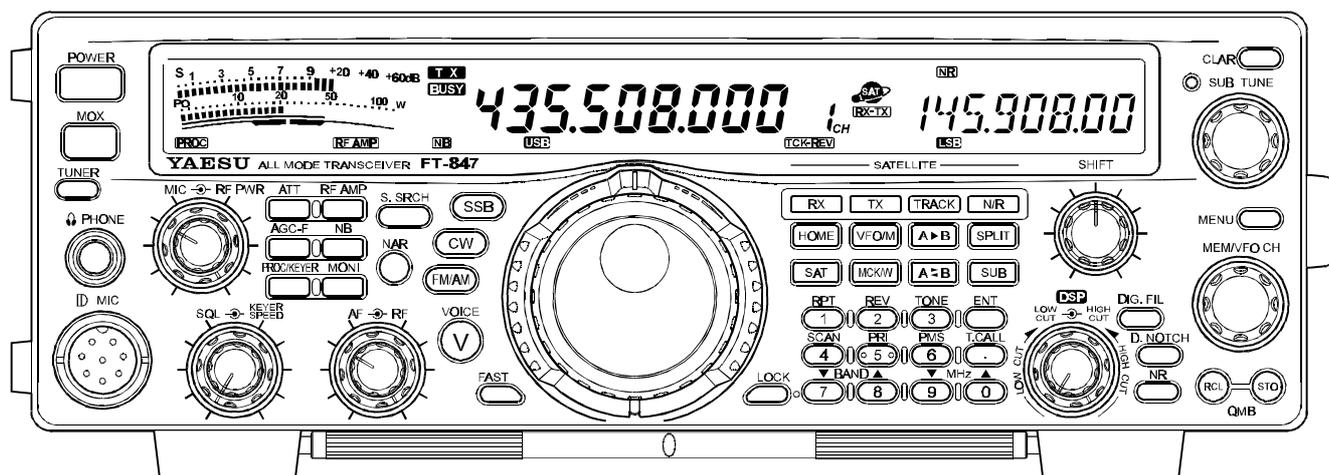
The exciting new Yaesu FT-847 Earth Station is a revolutionary multimode transceiver providing coverage of all nine HF Amateur bands, plus VHF/UHF coverage of the 50, 144, and 430 MHz bands.
