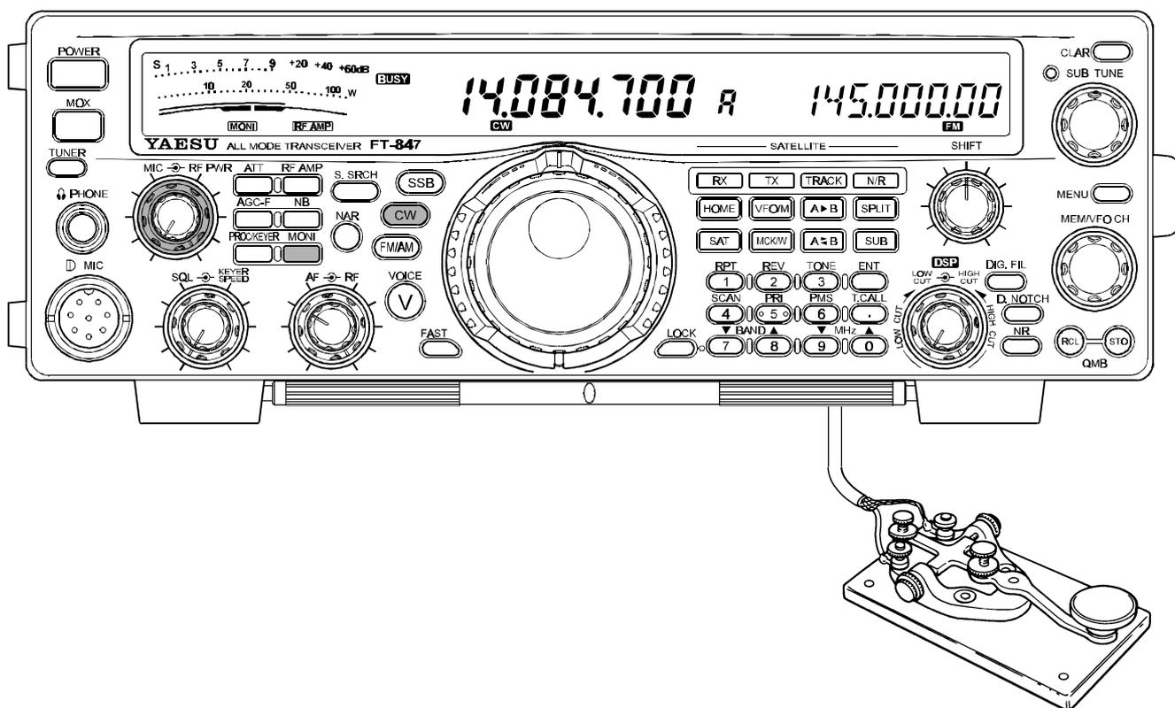
① Insert your key's ¼" three-conductor ("stereo") plug into the **KEY** jack on the rear panel of the transceiver. Remember that the Tip of this plug is the "hot" key lead, while the main shaft is Ground; the Ring is not used.
